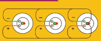
We encourage you to experiment with different configurations to see the effect. For example, you could put some MudWatts in series, and others in parallel and measure the circuits overall voltage and current values to see if they are what you would expect.
