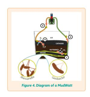
In a MudWatt, electrons are given off by the electrogenic bacteria surrounding the anode (the electrode that is buried in the mud). This creates a **higher concentration of electrons** at the anode than at the cathode so the electrons move through the wire towards the cathode.
